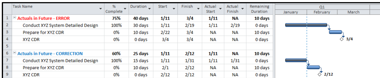
Figure 9.1.1-2 Impact of inaccurate Actual Start to Time Now and the Estimate to Complete (ETC)
