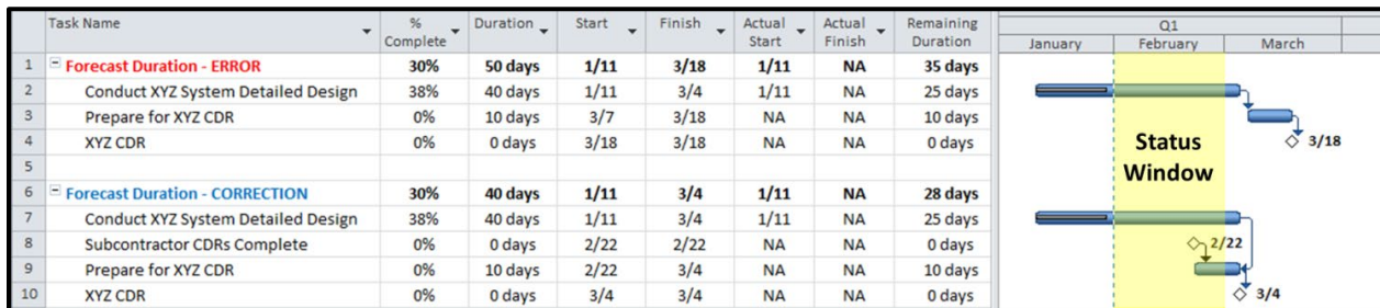
Figure 9.1.2-3 Example of a status that is missing a Logic Update outside of the Status Window
